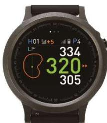
Press and hold button for
